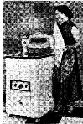
THE Swirlux model 504 de-luxe washing machine (Fig. 1) is a domestic cabinet model with 20½in. diameter tub taking up to 11lbs. dry wash in 12 gallons water. Tub is fitted with an improved design tangent-fin agitator which, it is claimed, provides greater water motion giving speedier washing and less buffeting with consequent reduction of wear on clothes.
