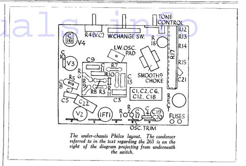
In some of the original receivers the condenser C21 of .05 mfd. connected between the anodes and cathode of the rectifier has been found to break down. This causes A.C. to be applied across the smoothing condensers C19 and C20, and as these are electrolytic the current passed is sufficient to blow the fuse.
