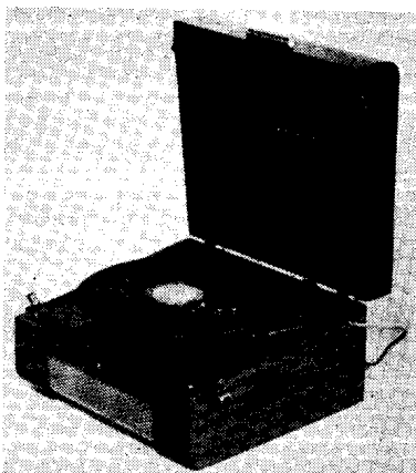
Electric record player consisting of a Garrard model S radiogram unit, fitted with a 10in. turntable, magnetic type pickup with automatic stop mechanism, and a two-valve amplifier, the output of which is fed into a 6½in. PM speaker. Designed to operate on 100-120, 200-250V 50c/s AC. Mahogany veneered table style cabinet. Made by McMichael Radio, Ltd., Slough, Bucks.
