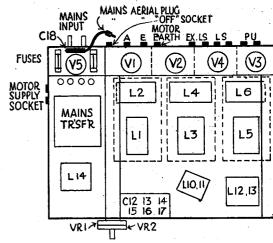
Ganging is carried out as is usual with simple TRF circuits by injecting a signal or tuning in a transmission of about 210m and adjusting the trimmers on the three sections of the ganged variable condenser for maximum output.
