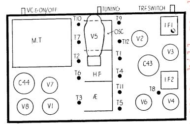
Two practical points to note with the 14/8 chassis is that two mains adjustments have to be made and withdrawal of the speaker plug disconnects the electrolytics.
