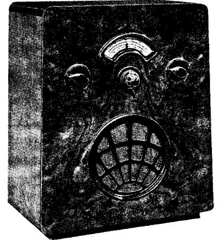
A five-valve Class B battery receiver the Duplex Transportable by McMichael Radio Ltd. is completely self-contained.
