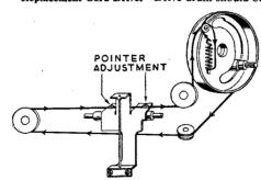
locked to gang spindle with the condenser set to its mechanical minimum (vanes unmeshed). With the drive cord fitted, the condenser should be rotated to maximum and the pointer carrier locked to the cord by the two clamp screws.
