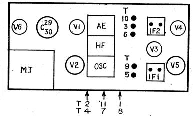
The diagram above identifies the valves and other main components on the top of the chassis and locates the trimmers, some of which are on the rear side.
