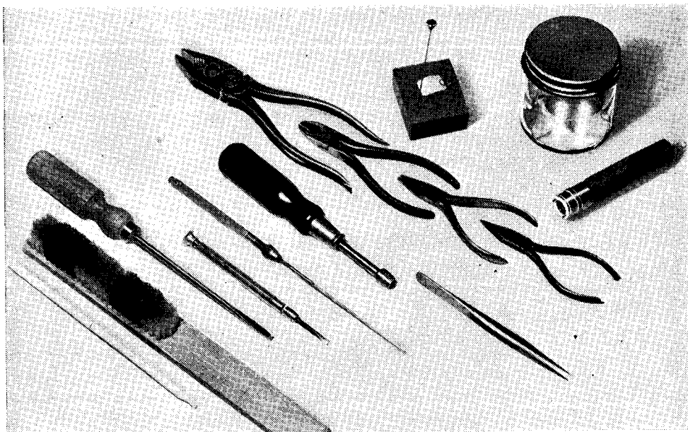
Your minimum clock repair kit. Left to right are, pegwood ; clock or typewriter brush ; clock screwdriver ; watch-maker's screwdriver ; reamer ; 6 BA box spanner and tweezers ; large pliers, cutters and two pairs of small pliers ; oil pot with dipper pin ; jar for cleaning fluid ; pin spanner (for dial nuts)
